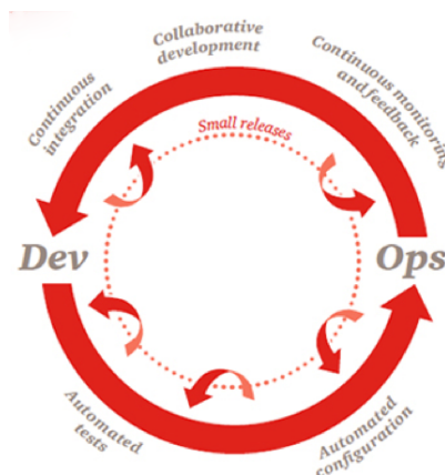
Figure 6.1: A DevOps work-flow connects development and operations in a continuous iterative process (illustration source: Gene Kim, HP, and PwC, 2013).
